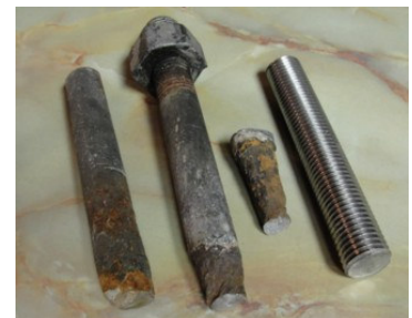
Samples of old bolts on the left, and piece of new stainless steel anchor bolt.
