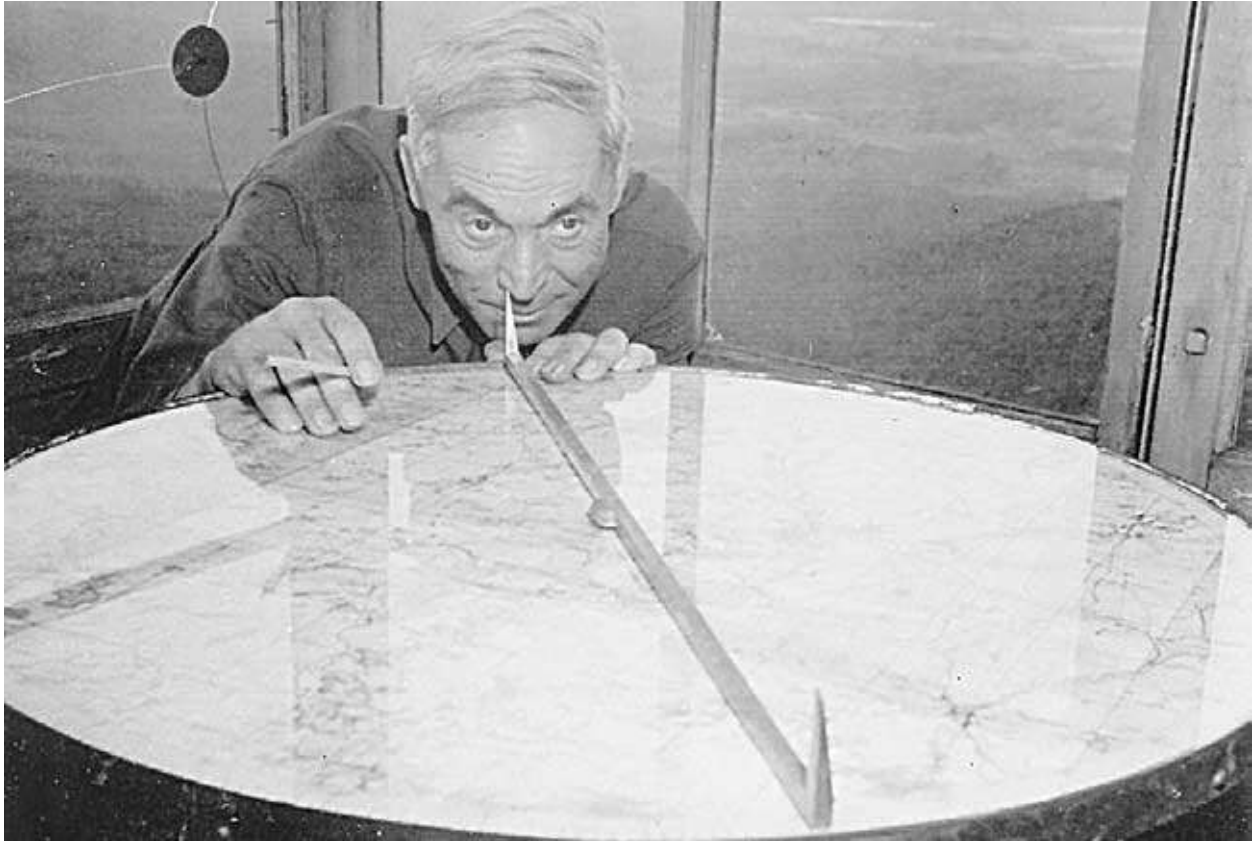
Hiram Denton, then the observer on Whiteface, demonstrates the use of an alidade, an instrument for determining the location of forest fires.
